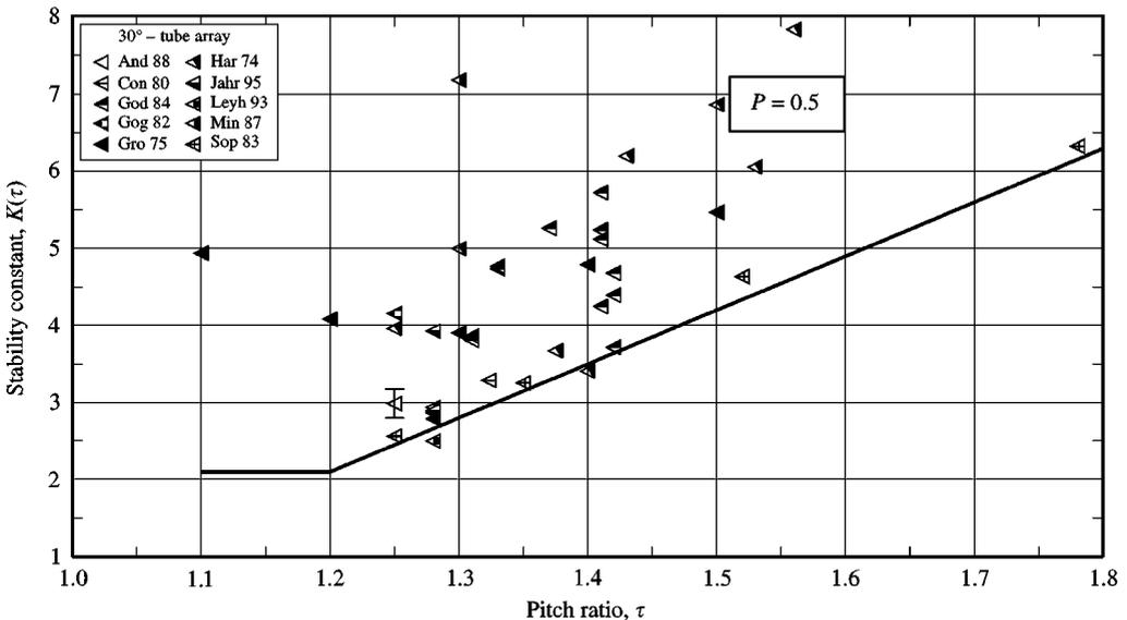
Figure 1. Effect of pitch ratio on the stability constant for gas flow and 30° tube arrays. The contractions in the legend as rather obvious and will not be elaborated; e.g. 'And 88' stands for Andjelic (1988), 'Con 80' for Connors (1980), and so on.
