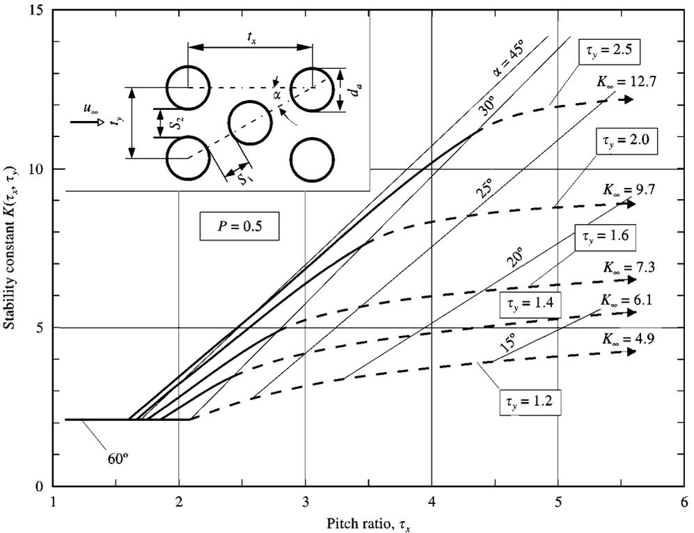
Figure 7. Stability constants for gas flow and non-standard staggered tube arrays.
