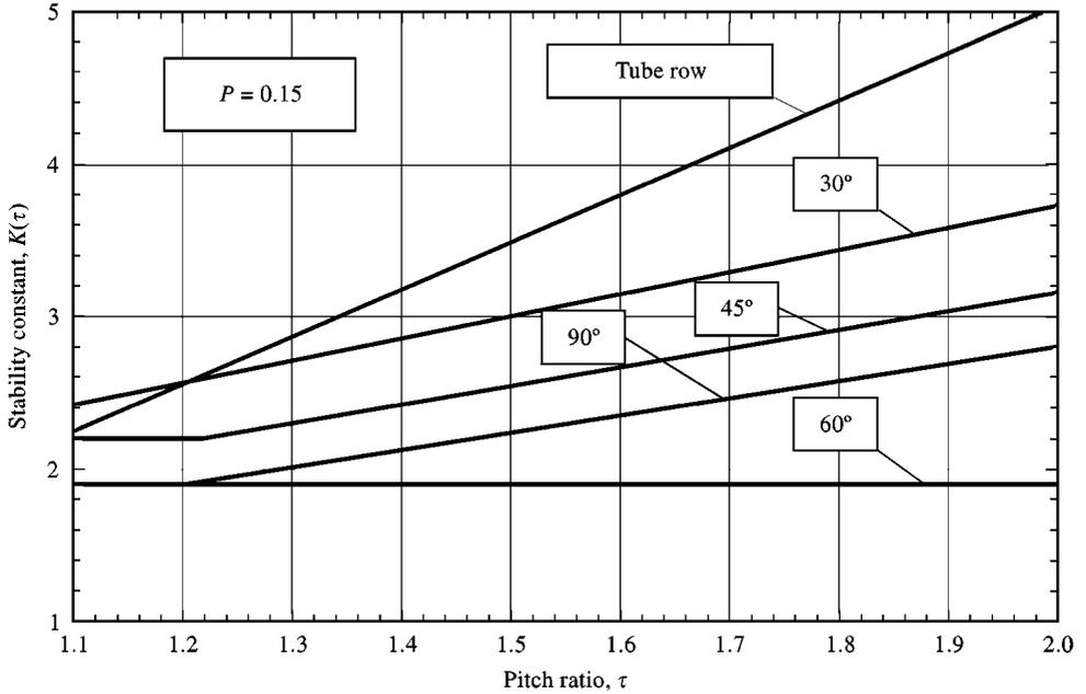
Figure 4. Dependence of stability constants on the pitch ratio for standard tube arrays and liquid flow.
