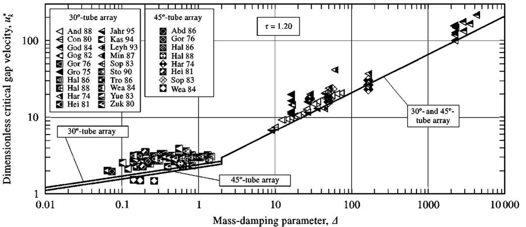
Figure 5. Stability map of dimensionless critical flow velocity versus mass-damping parameter for 30°- and 45°-tube arrays with  $\tau = 1.20$ . Refer to caption of Figure. 1 for meaning of contractions in the legend.
