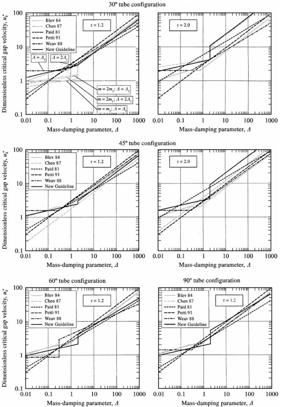
Figure 8. Comparison of design recommendations. Dimensionless critical flow velocity as a function of the mass-damping parameter.
