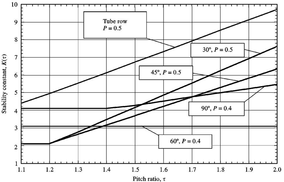
Figure 3. Dependence of stability constants on the pitch ratio for standard tube arrays and gas flow.
