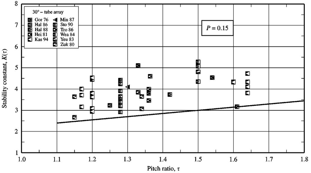
Figure 2. Effect of pitch ratio on the stability constant for liquid flow and 30° tube arrays.
