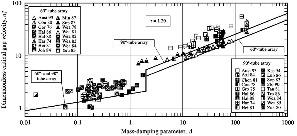
Figure 6. Stability map of dimensionless critical flow velocity versus mass-damping parameter for 60°- and 90°-tube arrays with  $\tau = 1.20$ .
